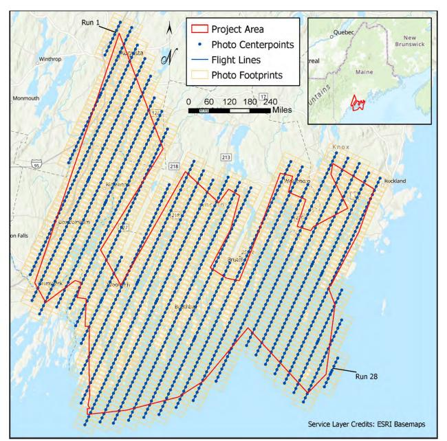
Figure 1. Flight lines, photo center points, and photo footprints for aerial flight photographs.
